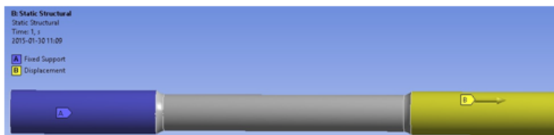
Fig. 7. Determination of fixed support (A) and displacement (B) on sample holders
